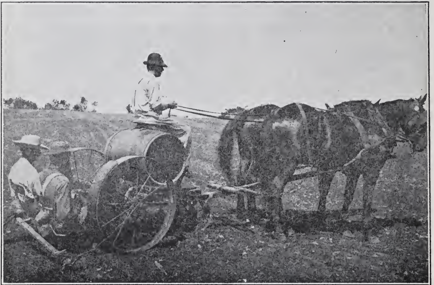
FIG. 4.—A type of tobacco planter commonly used in Pennsylvania.
